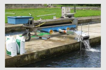
The fish counter is placed on his support tubes directly in a pond
